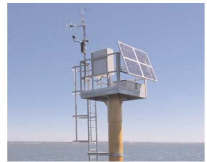
VPF-710 sensor as part of a weather station
