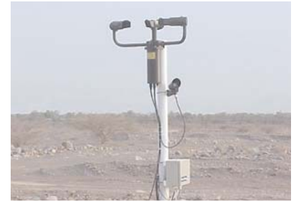
VPF-730 with Ambient light sensor
