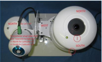
When mounting the Pyranometer, consider Northern or Southern hemisphere. The plug and cable always shall face "away from sun", to avoid heat by exposure to direct sun radiation, therefore likely corrupt Pyrano irradiance data.
