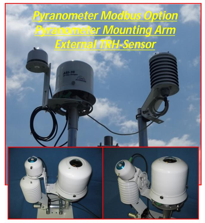
Pyranometer Option: To connect and operate a Pyranometer with any new ASI-16/51, for logging of real-time irradiance data (Act, AvP, AvM, Min, Max). Subject to purchase of Pyranometer Option. - Activation after Purchase.
