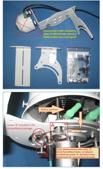
CMS ASI-16/51 "Pyranometer Mounting Arm" comes with two non-pre-assembled arm components, and small additional parts (screws, washers) for assembly and mounting. Screws to mount the Pyranometer itself are NOT included. Usual those screws are a part of the Pyranometer supplier scope of supply.
