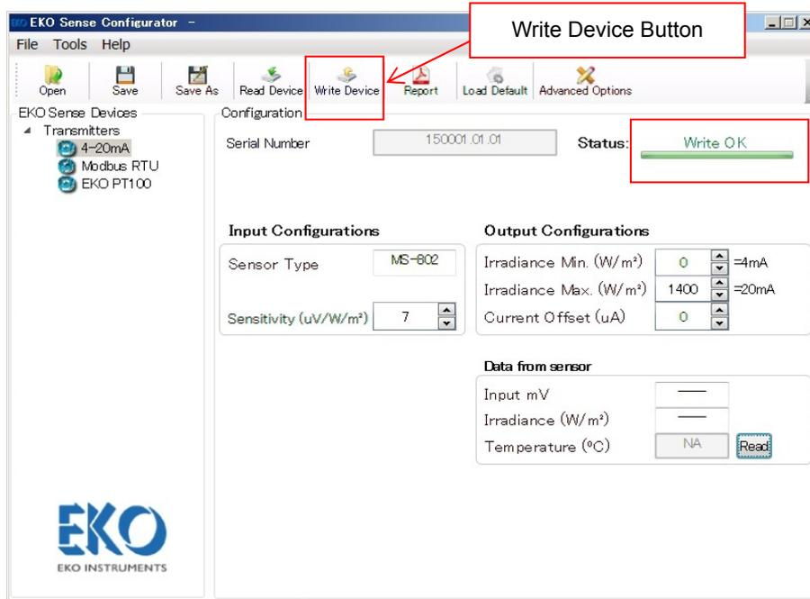
Figure A-13. Write Device Button
