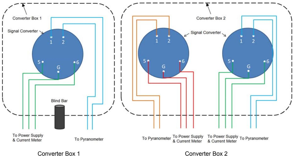
Figure A-22 Wiring Example of Converter Boxes
