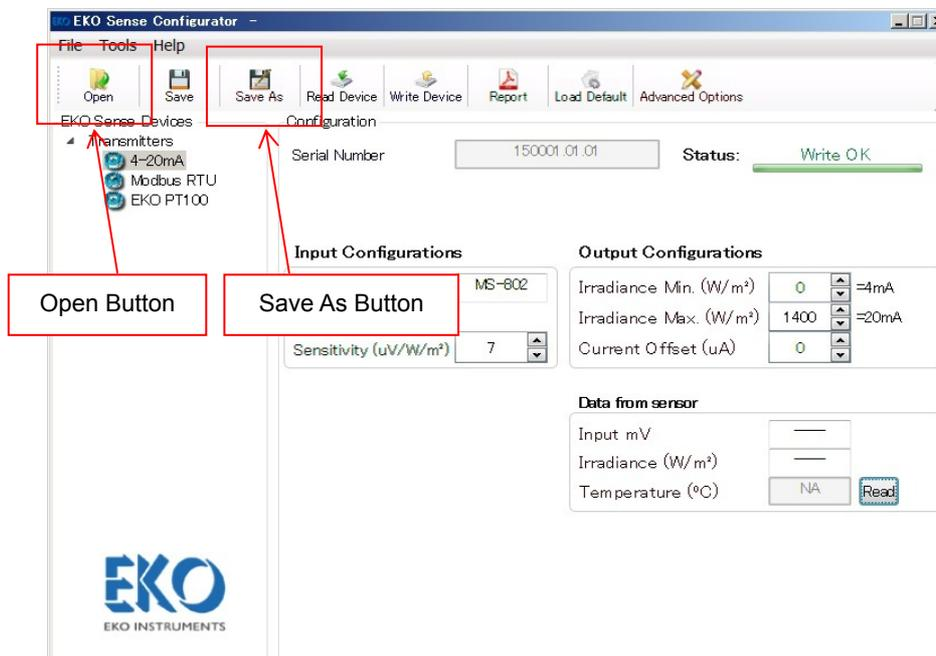
Figure A-14. Save and Load Configuration
