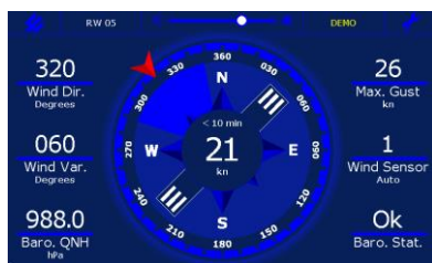
Display for wind/meteo on airfields. Wind information is shown relative to the north as well as to the runway. Runway heading may be adapted (during installation), while parameters are indicated conform ICAO regulations.
