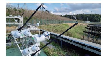
Designed for scientific research, industrial applications, and photovoltaic system performance monitoring, the MS-40, with EKO's universal sensor design assures best in class accuracy, speed and reliability whatever your application.
