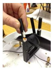
Figure 6 - SBS replaceable reed switch (left) / Empty socket to house one of the reed switches (centre) / reed switch being inserted into the empty socket.
