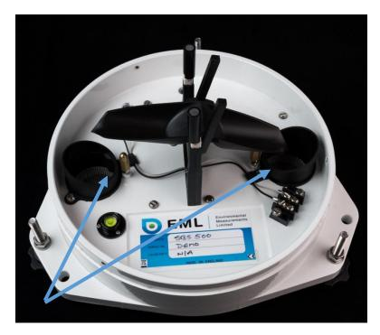
Figure 5 - Internal photograph highlighting water drains
