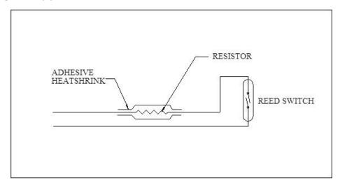
Figure 3 - Reed switch and resistor
