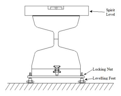
Figure 1 - Levelling the Gauge
