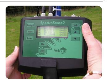
Multichannel meters for Light Sensors
