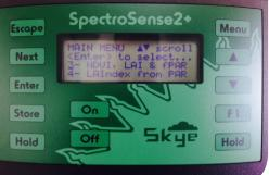
Logging display meter for visible/NIR light sensors Incident & reflected light measurements Matched to satellite wavebands Direct readout of NDVI Logging of measurement location
