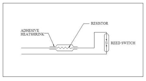
Figure 4 - Reed switch and resistor
