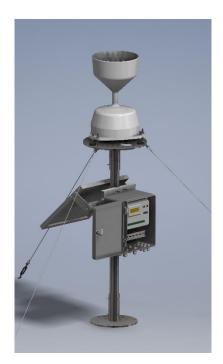
Figure 3 – Rain gauge fitted to a pedestal as part of the EML system
