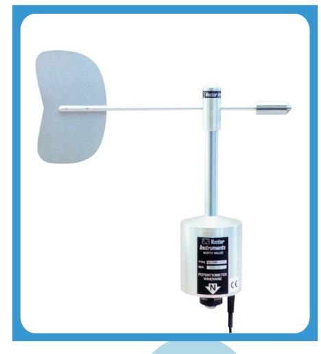
A precision wirewound potentiometer mounted in the same all-weather.. corrosion resistant case as the Porton Windvane. The potentiometer has the lowest possible torque consistent with long life and reliable cperation. The small gap at North is filled with an insulating material to ensure smooth operation over the full 360°. The vane arm is attached by a unique gravity fastener, giving rapid and reliable attachment and release in portable applications.
