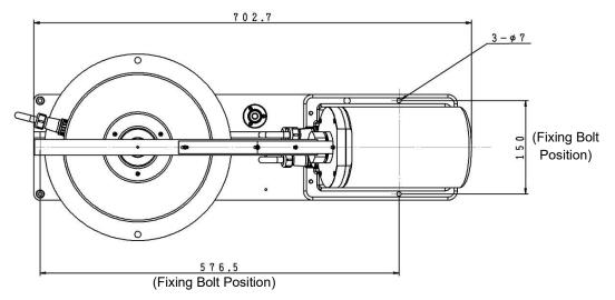
Figure 5-3-2. Location of the Holes for Fixing Bolt
