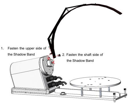
Figure 5-3-3. Fixing the Shadow Band
