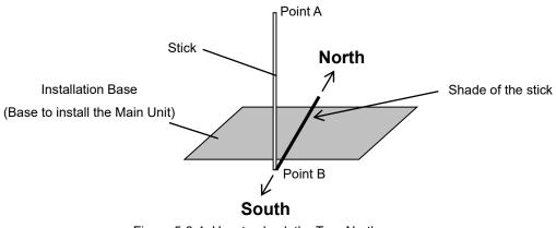
Figure 5-3-1. How to check the True North (shade is shown in true north side at culmination time)
