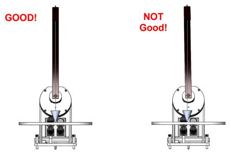
Figure 5-3-4. Fine-Tuning the Tilt on Shadow Band
