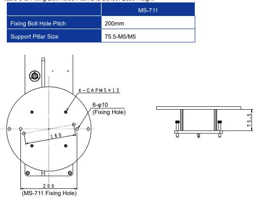
Figure 5-3-5. Fixing Holes for Spectroradiometer
