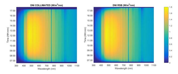
Fig. 4. DNI measurements with collimated spectroradiometer (left) and estimated DNI with RSB spectroradiometer (right)
