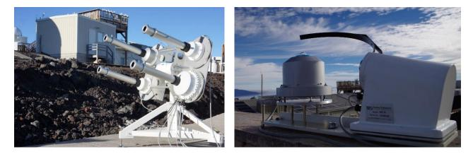
Fig. 1. Left: MS-700, MS-710, MS-711 and MS-712 mounted on an EKO STR-32G tracker; Right: EKO MS-711 mounted with the RSB-01S rotating shadowband.
