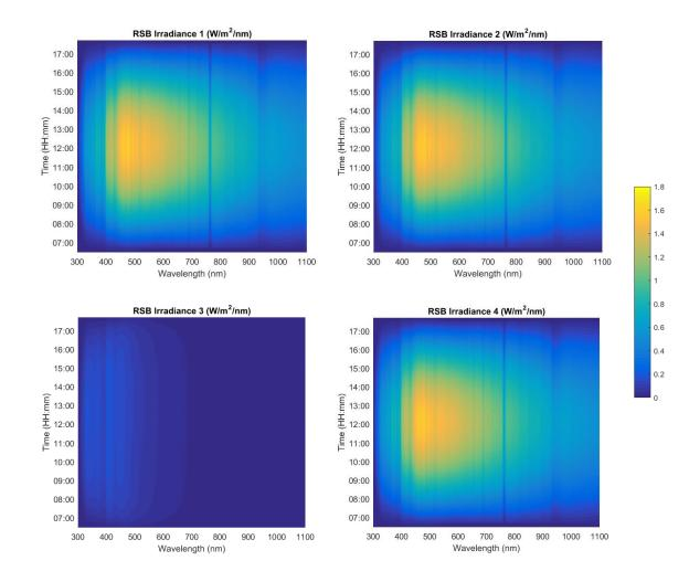
Fig. 3. RSB spectroradiometer measurements at different positions: 1<sup>st</sup> position GHI, 2<sup>nd</sup> position band at -5 °, 3<sup>rd</sup> position DHI, 4<sup>th</sup> position band at +5°
