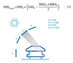
Fig. 2. Rotating shadow band sweeping positions
