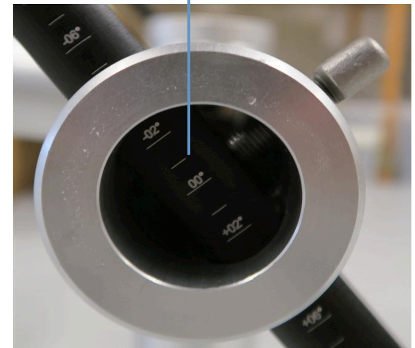
*Before installing the detector itself the detector-adjusting bar has to be shifted to an initial position. The easiest way to achieve this is first to set the shadow ring sliding bars to equinoctial position (declination  $\delta = 0^\circ$ )*
