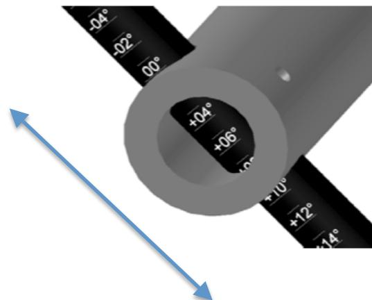
Declination values throughout the year are indicated on the next slide. The bar need to be adjusted on a weekly basis.
