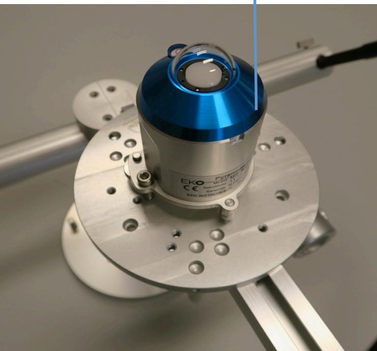
*Install the pyranometer with the 2 bolts.*
