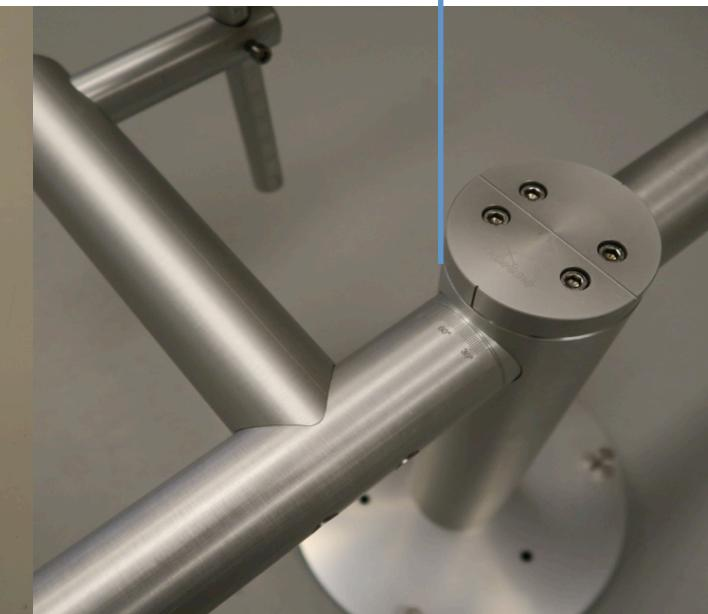
*Attach the radiometer cross bar.*
