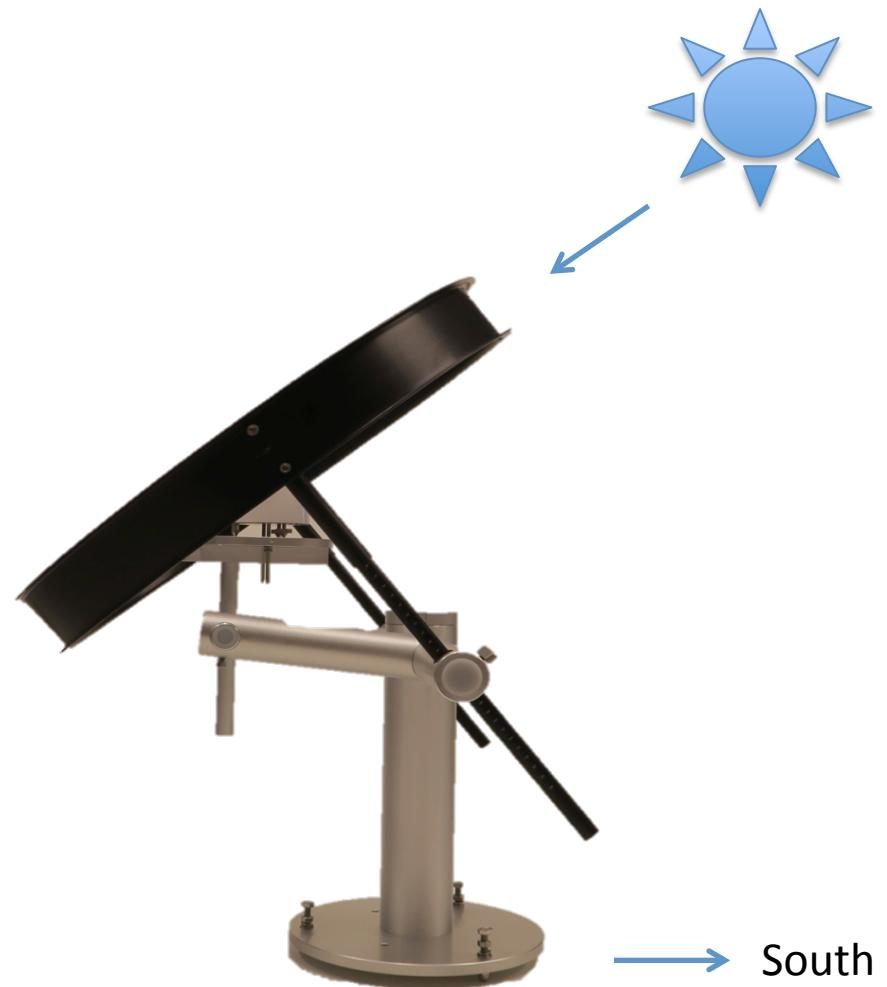
The mounting base of the RSR-01 should be placed in **horizontal position (leveled)** and **true North/South orientation**.
