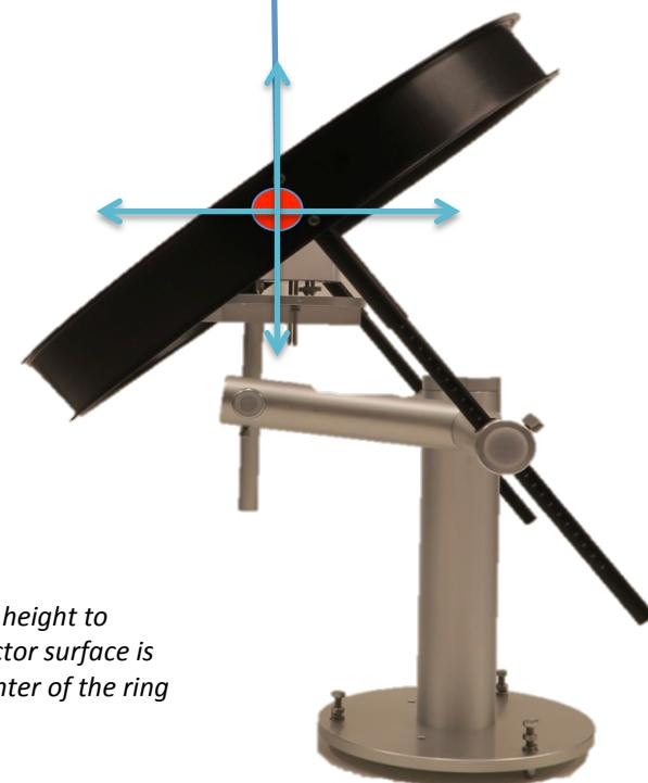
*Adjust the sensor height to position the detector surface is position in the center of the ring (y)*
