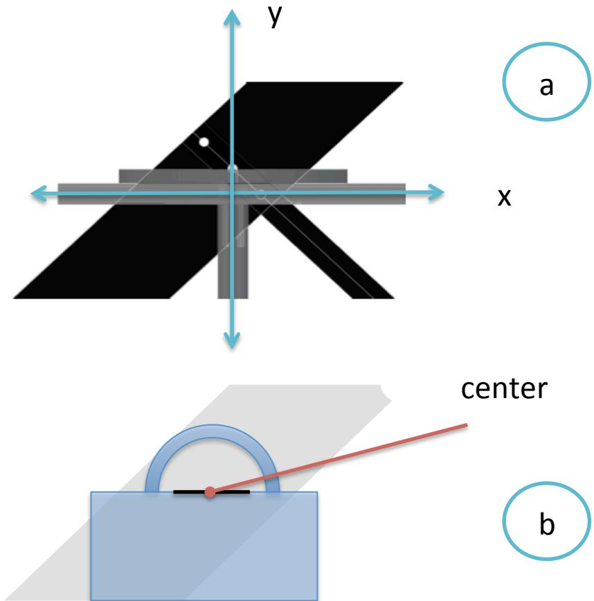
Shown in illustration (a) the mounting plate is taken as reference. The top of the mounting plate can be moved in  $x$  and  $y$  direction. When the sensor is already mounted, illustration (b), take the black surface as a reference.
