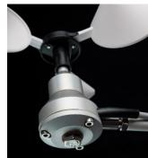
The wind speed sensor consists of a low-inertia ABS cup assembly for fast response mounted on a dual ballrace-supported stainless steel shaft. The use of a magnet operating a long-life reed switch produces one bounce-free pulse per revolution of the rotor.
