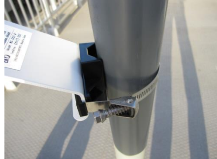
Figure 4-8. Mounted on a Pole
