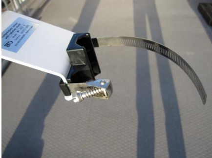
Figure 4-7. Before Fastening Band
