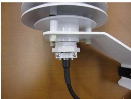
Figure 4-5. Insert Temperature Sensor
