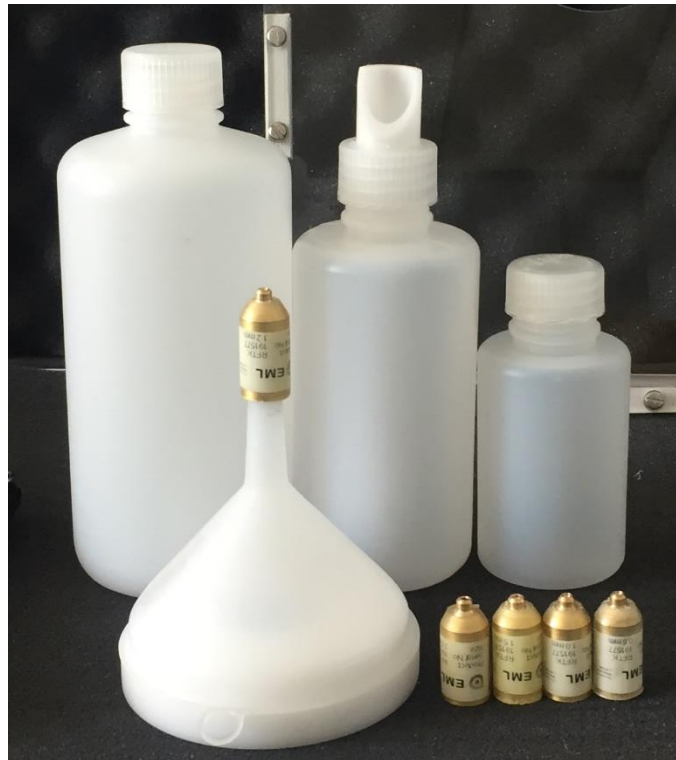
Figure 2 - Three bottles, five brass nozzles, plastic funnel, acetal ring and special acetal bottle-nozzle, comprising the majority of the field verification kit.
