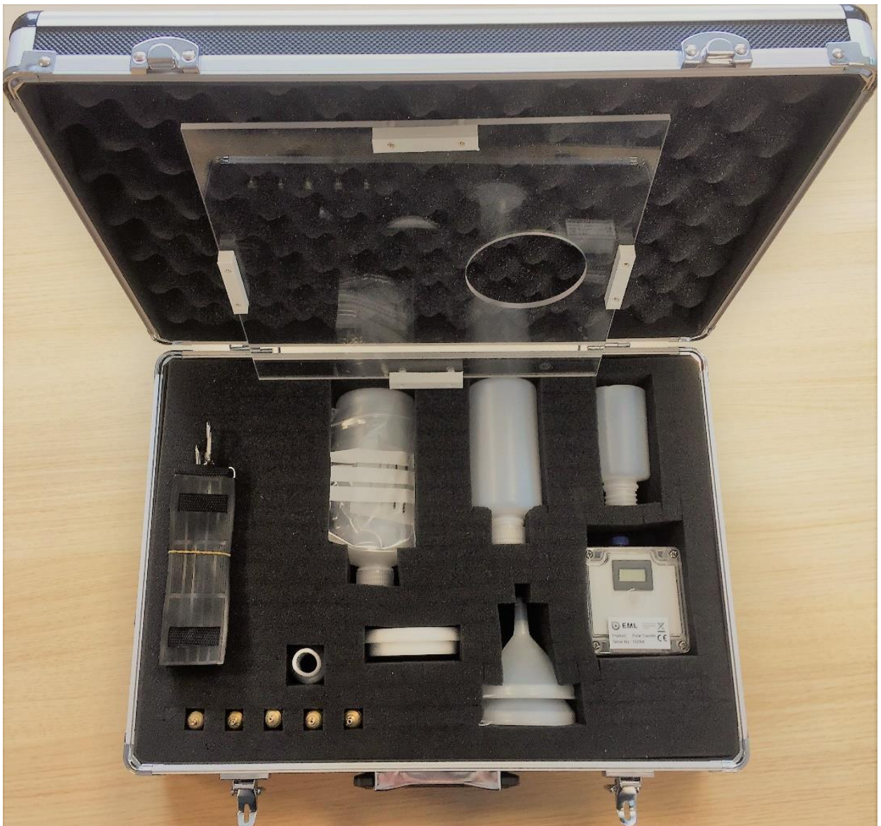
Figure 1 - The EML Rainfall Intensity Field Verification Kit (P-780-650) with Pulse Counter (P-780-630), The two items, the field verification kit and the pulse counter, are available separately.
