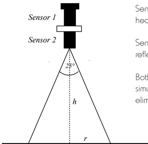
Sensor 1 is fitted with the cosine correcting head and is measuring incident light.
