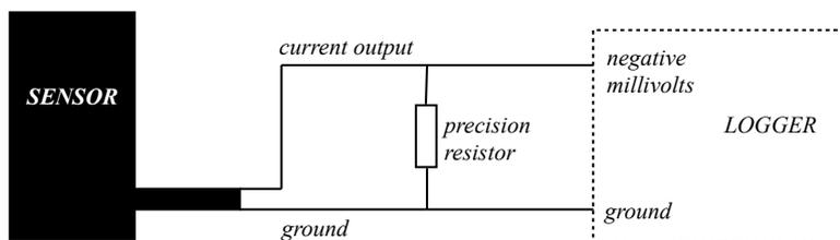
The millivolt signal will be proportional to the current output and resistor value as shown:
