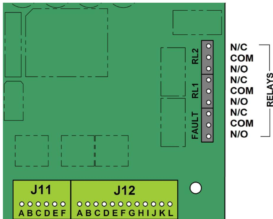
The relay connections are along the right-hand side of the main circuit board at the cable gland end. The connections are a two-part connector with pins in the circuit board and a removable plug for the connections. It is advised that the removable plug is removed from the pins (pulled upwards) to enable the connections to be made to the cable before re-connecting to the circuit board. The connections in the removable plug are of a screw clamp type.
