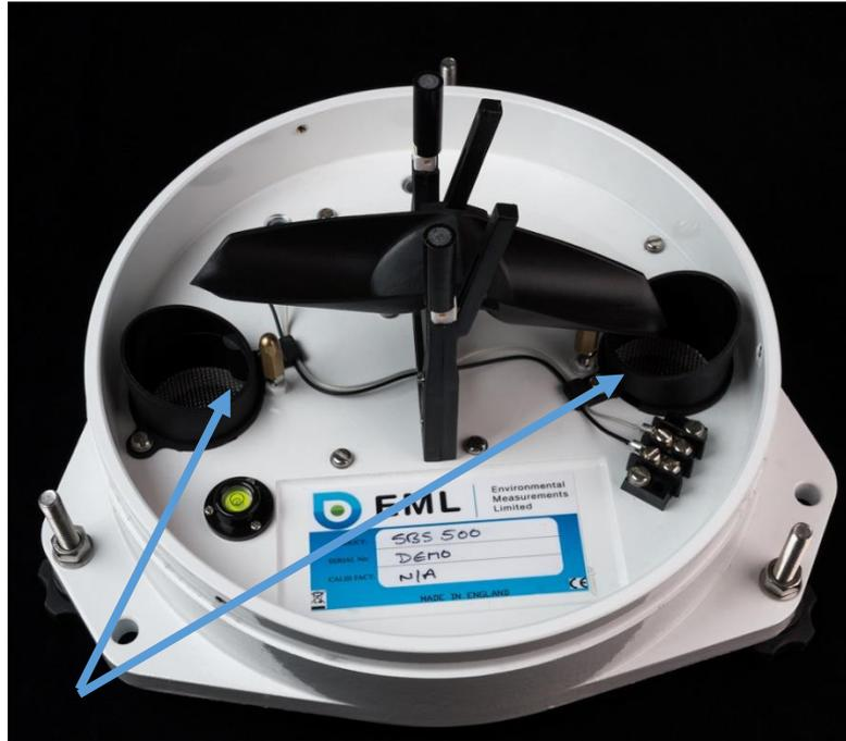
Figure 5 - Internal photograph highlighting water drains
