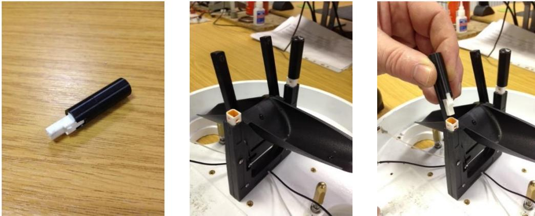
*Figure 6 - SBS replaceable reed switch (left) / Empty socket to house one of the reed switches (centre) / reed switch being inserted into the empty socket.*
