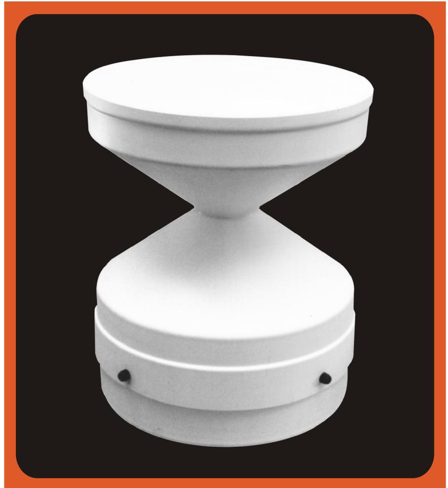
A conventionally shaped rain gauge interferes with the airflow so that the catch is reduced. The low cost ARG100 aerodynamic gauge has been designed to minimise this effect by presenting a reduced area to the wind. The profile is very similar to that derived theoretically and independently by the U.K. Meteorological Office as an 'ideal' shape.
