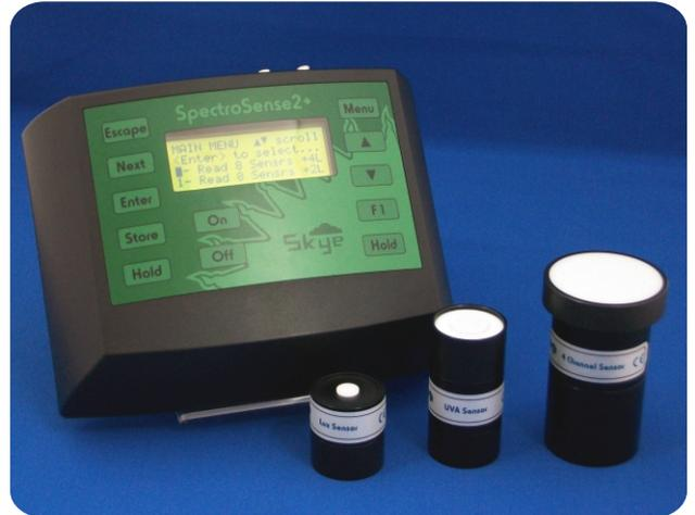
Logging display meter for visible and NIR light sensors
