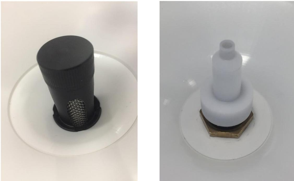
*Figure 5 - Filter and filter cap (left) / Nozzle delivering water into tipping bucket (right)*
