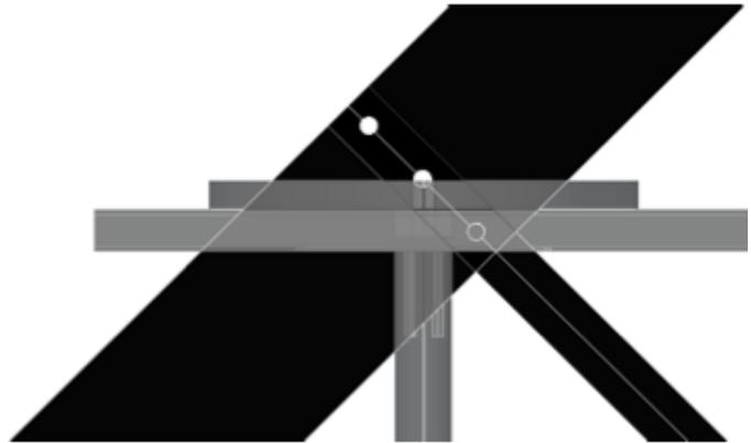
horizontal alignment, loosen the detector-adjusting fixation so the detector base plate is free to slide on the detector-adjusting rail (if the RSR-01 is used on a site near the equator or near the poles the possible displacement offered by the length of the detector-adjusting rail is not sufficient. In that case this rail has to be mounted eccentric in the necessary direction).
